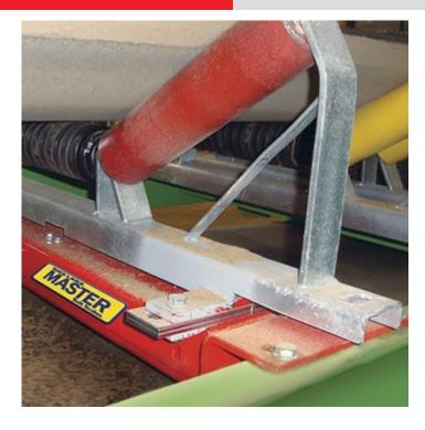
The BS311 MASTER belt scale weigh frame is suitable for medium to heavy capacity belt conveyors. Easy to install and in standard or custom made dimensions, it easily fits on the conveyor frame by using only four bolts.
